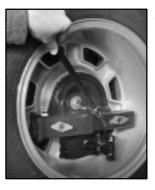
Place the end of the spanner wrench on the nut and then turn the wheel wrench counterclockwise to loosen the nut holding the tire to the carrier.
